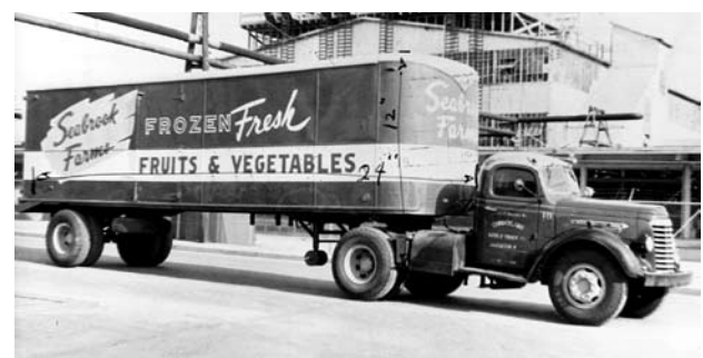
Pictured is one of the many tractor trailers owned by Seabrook under the name Cumberland Auto & Truck Co. It was an early version of the refrigerated tractor trailers used for frozen food delivery.
