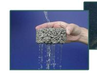
Porous concrete (above right) looks like the concrete you're used to, but rain and snowmelt filter right through (above). Concrete can be shaded with earthy tones for a more natural appearance.
